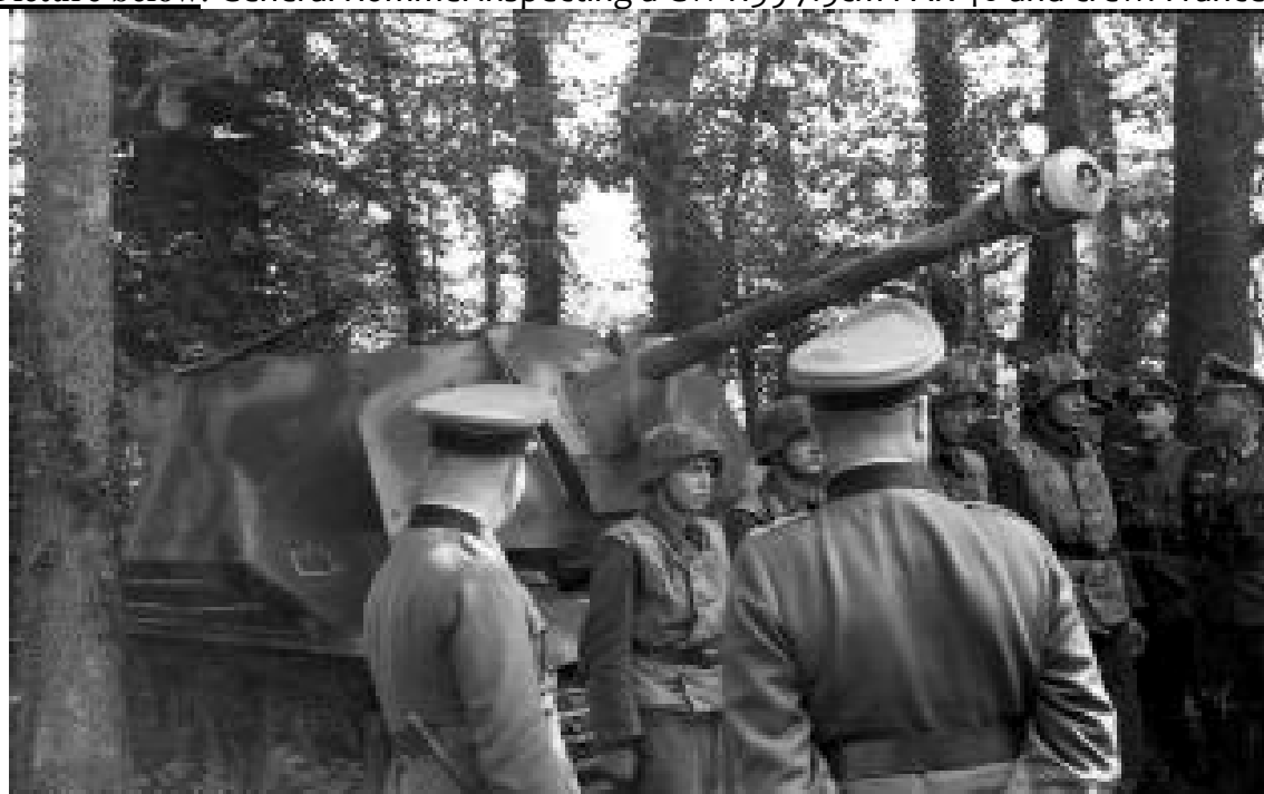
Picture below: General Rommel inspecting a GW H39 7.5cm PAK 40 and crew. France
